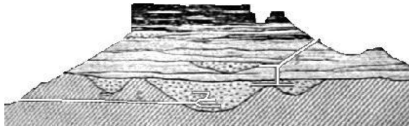
Figure 5.12. Side view of Table Mountain, Tuolumne County, California, showing mines penetrating into Tertiary gravel deposits beneath the lava cap, shown in black (Holmes 1899, p. 450).
